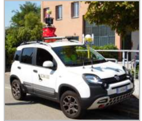
Configuration of use with FARO LASER SCANNER
